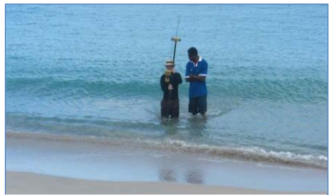
Figure 2: High Resolution Coastal Profile Surveying with GPS
